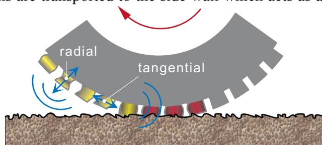
surface. The stick-slip mechanism is normally associated with situations where relatively high tangential forces are applied to the tyre (e.g. acceleration, braking, cornering). The role of this mechanism for free rolling conditions is unclear.
