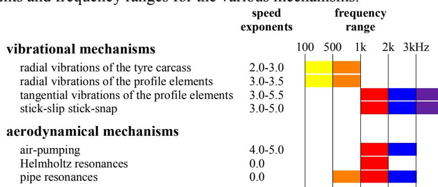
Figure 1: Overview of speed exponents and frequency ranges for tyre/road noise generation mechanisms.
