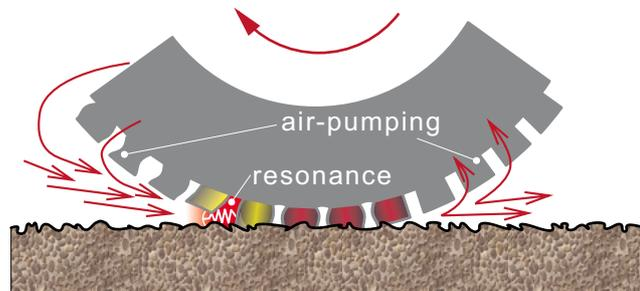
*Pipe resonance.* Each tread pattern, in contact with a rather smooth road surface, constitutes a system of pipe resonators. Their resonant frequencies depend on the geometrical properties but not on the rotation speed of the wheel.
