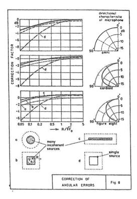
From the results it can be seen, that the situation d entails the greatest correction which typically amount to
