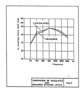
This figure gives a comparison of the measured and the calculated im-. mission level of an existing plant. The difference between measurements and calculations are for all octave bands smaller than 2,5 dB. The difference in A levels is typically smaller than 1,5 dB.
