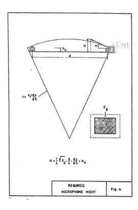
For most practical applications the radius of the downwards bent sound ray is approximately equal to 5 km and with the distance (d) equal to 2 km, one obtains for the relevant emssion angle
