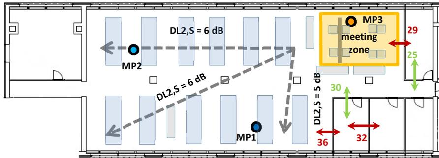
Fig. 2. existing office plan with measurement positions and results.
