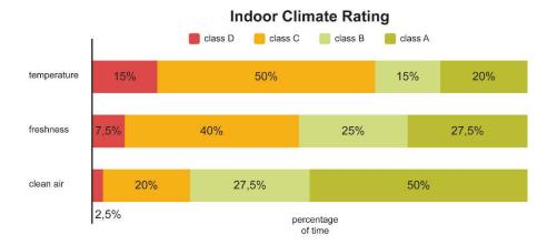
display ICR per component -distribution of measurement results into comfort classes
